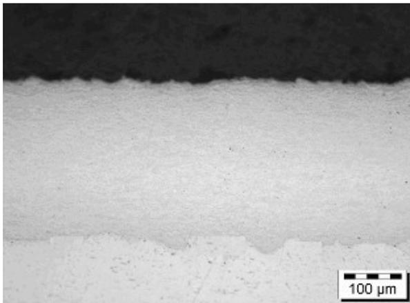
WC-CoCr spray coating on unalloyed steel
