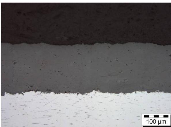
Zirconia spray coating on unalloyed steel
