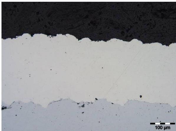
Coating NiCr on low carbon steel St37-3
